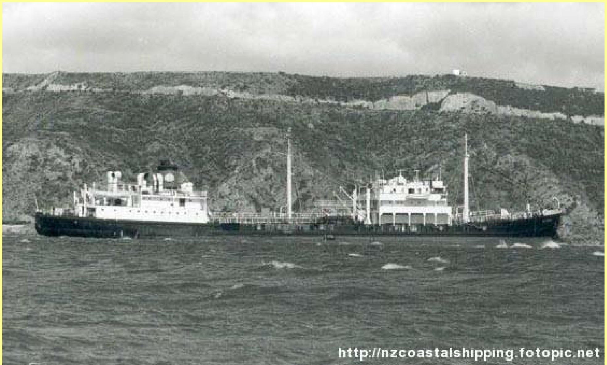
MAUREA. 2,926grt. 331' 11" x 46' 4" x 17'. A specially built bitumen tanker
